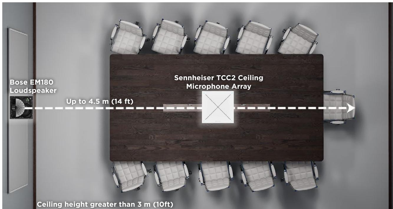
**Microphone Array:** The Sennheiser TeamConnect Ceiling 2 provides a patented automatic voice location detection and dynamic beamforming to capture a presenter's voice no matter where they are located in the room. It quickly switches between multiple voices and it's great for rooms with flexible seating configurations.
