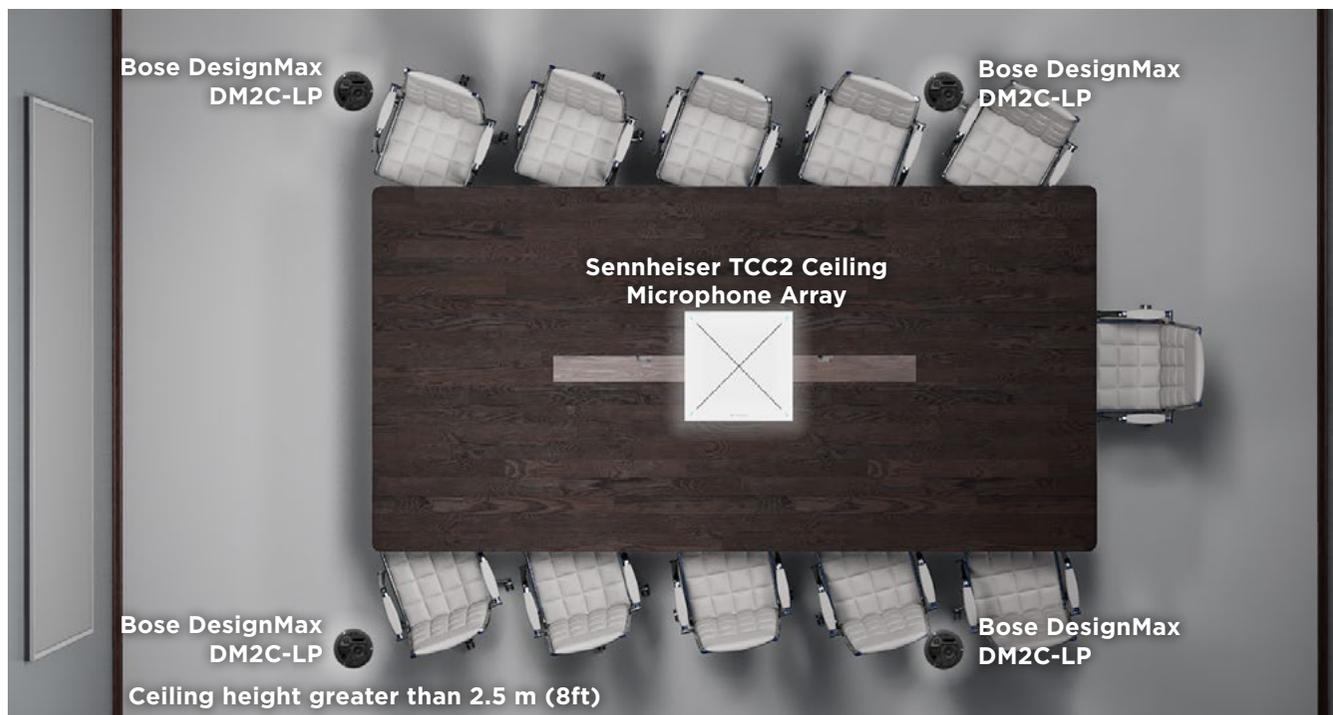
**Microphone Array:** The Sennheiser TeamConnect Ceiling 2 provides a patented automatic voice location detection and dynamic beamforming to capture a presenter's voice no matter where they are located in the room. It quickly switches between multiple voices and it's great for rooms with flexible seating configurations.
